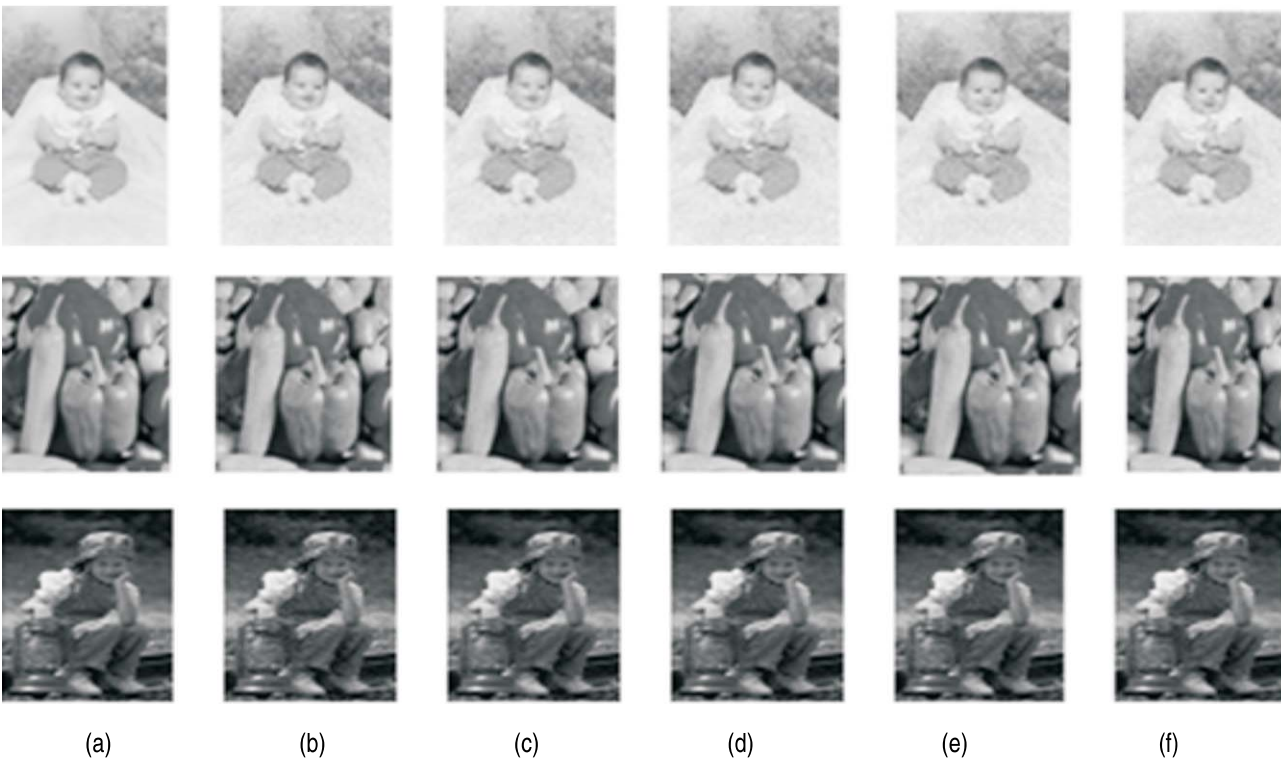
Fig. 51. Baby.jpg, pepper.bmp, girl.jpg (a) original image (b) Zero mean and 0.9% variance Gaussian noise (c) images restored by SMF (d) images restored from by TDF (e) images restored by CWF (f) images restored by proposed algorithm
